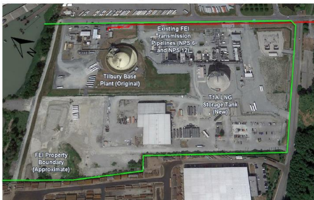
Figure 1: FEI Existing Assets, Tilbury Island, Delta, BC
